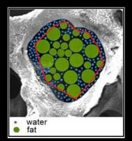
"Water is more prevalent in the boundary zone while fat occupies primarily the central zone of the pore"
