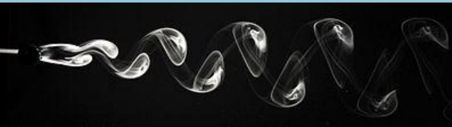
vortex street behind a circular cylinder in air; the flow is made visible through release of oil vapour in the air near the cylinder
